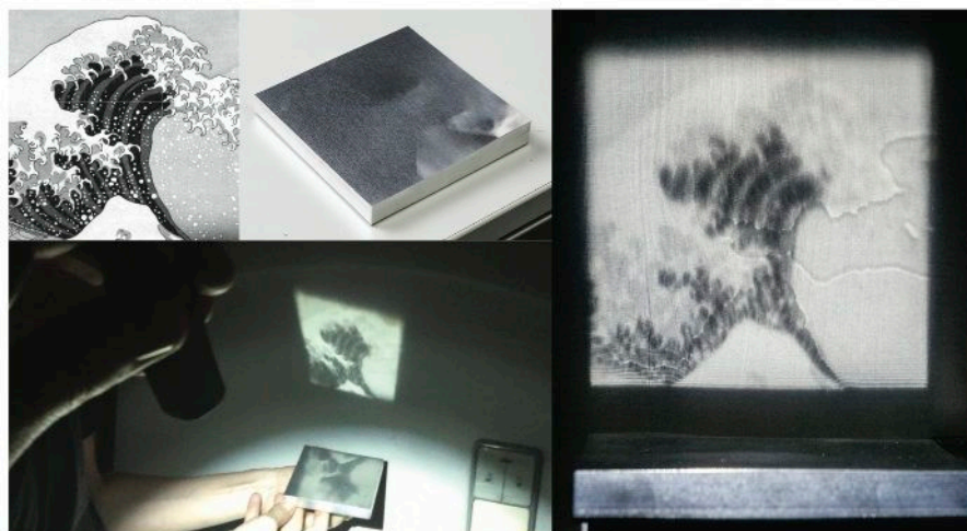
The target image (top left), the aluminium mirror (top middle), and the reflective caustic from the polished version.
