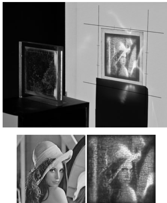
The experiment ( top ), target image ( lower left ) and experimental result ( lower right ) for the caustic imaging achieved in the Zurich Disney Research lab.
